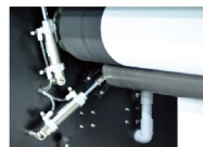
LEVEL MEDIA ROLL Decreasing wrinkles during substrate's feeding and raising the friction of main roll for smooth feeding operation for all kinds of fabrics.
