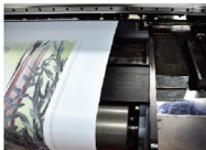
POST HEATR Adjust two post heaters for better dry efficiency.
