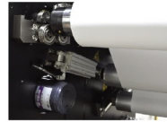
DANCER BAR It can maintain constant media tension to secure stable feeding.
