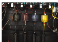
AIR DEGASSING UNITS It removes micro bubbles in ink while transferring ink to main ink tank.
